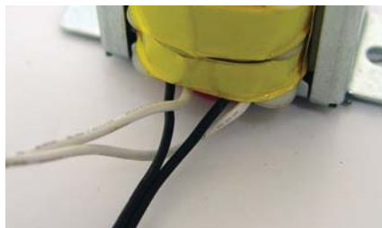
Both black wires go to switch and both white wires go to the neutral - power cord white
