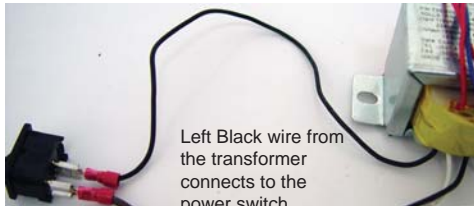
Right side White wire from transformer connects to the Blue - NEUTRAL power cord.
